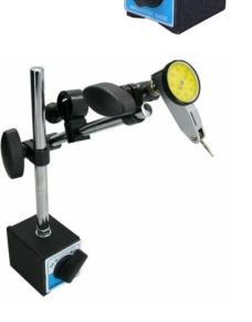
An alternative gauge is the lever arm type shown here. The version I have has the same range and resolution as the previous version but the plunger moves from side to side rather than in and out.
