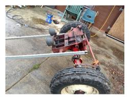
The tombstone is bolted to the engine by 4 bolts (one is longer than the others.) The engine and all behind it need to be supported so these bolts can be removed and the front axle assembly wheeled away. There are a couple of ways this can be done:
