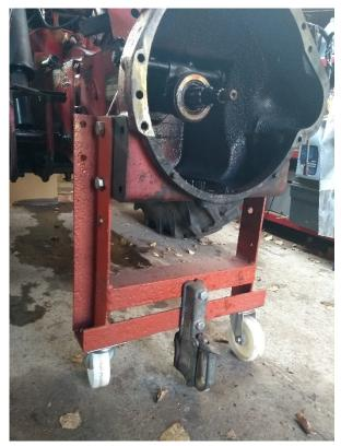
guess trying to pick the balance point but the engine is tail heavy due to the flywheel and clutch. A rough guess is with the crane about 2/3 of the way along the leveller towards the back wheels.
