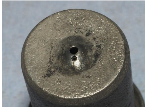
Nozzle from a BMC 1500 engine. Note the smaller pilot hole to squirt fuel onto glowplug and the radial crack through both holes.
