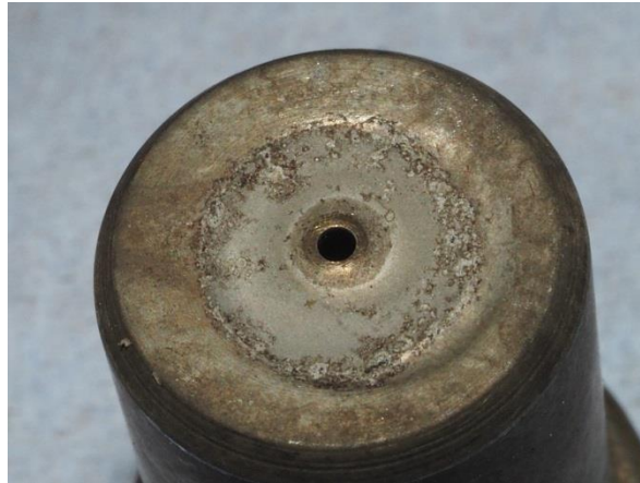
Nozzle from an International Harvester BD154 engine in a B414. This is in relatively good condition – at least from the outside.
