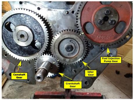
on each of the gears, highlighted in this case by yellow marker pen. Actual setting of the timing will be covered in a later article when they are re-assembled.
