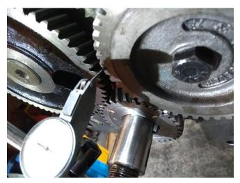
A dial gauge can also be used. Here the gauge is measuring the camshaft gear looking through the hydraulic pump mounting hole.
