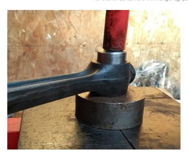
This picture shows the old bush being removed. The insertion tool is used to press out the old bush which slides into the outer support. My little 6 tonne press had no difficulty pressing the bushes out.
