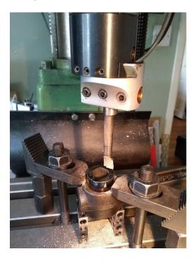
An alternative to the reamer is a micrometer boring head. Being much shorter than the reamer and a single point cutting tool, its centring in the hole is significantly more accurate. I sharpened the carbide tip on a diamond hone to give a very fine edge. Using several spring passes after each adjustment I increased the hole size to achieve the "a little tight" fit.
