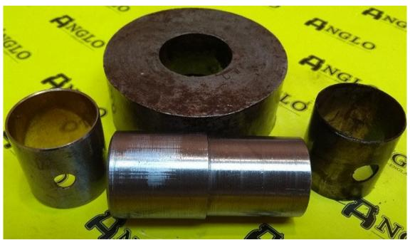
Replacing the bushes is relatively straightforward, but they will have to be finished to size once inserted.
