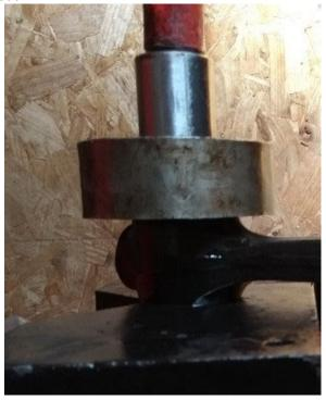
This photograph shows the insertion setup. I oil the bush (inside and out) and the con-rod hole. The actual bush is inside the support tool and just about to be pressed into place.
