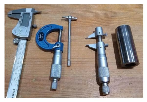
While measuring the piston pin with a micrometer accurately isn't too difficult, measuring the bush's bore is more challenging. This photograph shows the most likely options is the home workshop:
