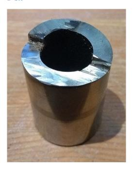
D-bits are often used for drilling flat bottomed holes but are also good for deep and/or accurately sized holes. An internet search will provide many examples of how to make them.
