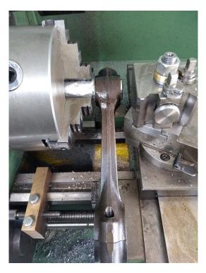
While still within tolerance, the new piston pins were slightly larger (about 1 thou) than the old pins. The new pins were therefore used to prove the final fit in the bushes and help improve the bushes' surface finish.
