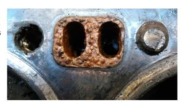
From new these engines use Helicoils in the block as standard, so the bolt screws into the Helicoil which in turn had been screwed into the block.
