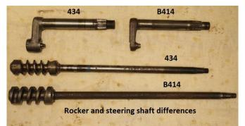
The rocker shaft pin is the main point of wear in the earlier steering box. This photograph shows how much heavier the rocker shaft is around the pin in the later design although the tip of the pin is actually smaller.
