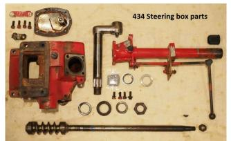
on my 434 appears to be a service exchange unit by the label (the tag top left of the picture) but was actually missing one of the ball bearings, presumably missed when factory reconditioned.
