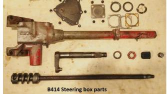
above and one below the steering shaft worm. The bearings should be held in a cage, one of which had totally disintegrated in this box.
