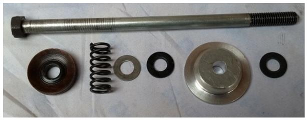
This picture shows the retaining screw and associated parts. No O-ring (10) was fitted so I'll have to find something when it is re-assembled. As the element guide was missing and I had no reference model to work from, I made a replacement from a piece of aluminium that I had around to replace the original pressed metal part. Interestingly there was no groove for the (missing) circlip (4) so I've used a rubber washer for the first trial but finally fitted a circlip into the end of the thread.
