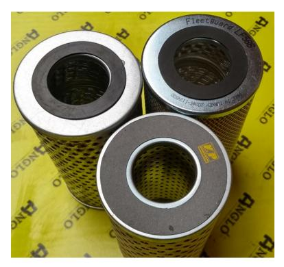
These are the same cartridges showing the sealing disk on the end. A similar seal is on the other end and so they can fit either way up.
