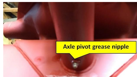
Figure 6 Underside of front axle showing the important grease nipple
