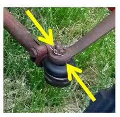
The two hammers are simultaneously swung at opposite sides of the arm holding the taper as shown by the arrows in this picture.
