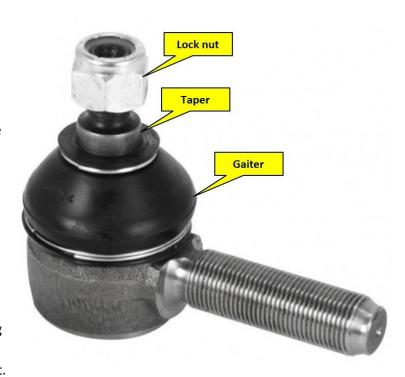
If the lock nut and/or thread are damaged and we release the taper, it will not be possible to further undo the nut.
