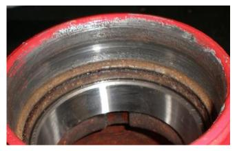
The bearings are simple press fit and the photograph shows one of two notches under the outer bearing shell where the shell can be knocked out with a punch.
