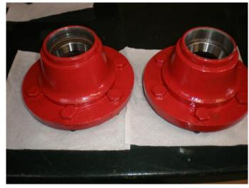
can make them slack. If the threads aren't kept clean and free (personally I assemble with a little copper grease) then the bolts end up turning in the hub when removing the wheel and wearing the fit so the problem gets worse. Some people even revert to welding on steel bars to join all the bolts together to stop them turning! A better solution would be to remove the bolts and add a little weld to one of the flats so when it is refitted it can't rotate.
