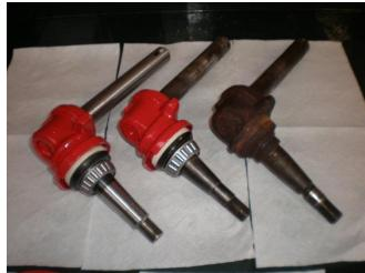
The final insult with this knuckle came when the tractor was driven out of the workshop – the tractor would only turn right, not left. The forging was of such poor quality that it had to have quite a lot removed with the angle grinder before it would turn in the other direction.
