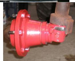
One final point when rebuilding the steering knuckle is to get the lip seal the correct way round. Its purpose is to keep dirt out of the hub, NOT to keep the grease in.
