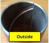
Tolerances on the early original bushes required them to be reamed to size once inserted but the modern parts don't seem to need this. Supplies change so reaming may however be necessary. The kingpin part of the steering knuckle should rotate smoothly but there should be <u>NO</u> side to side movement.
