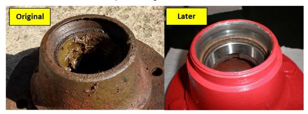
In the past I've modified the earlier hubs to take the lip seal by adding an extra sleeve as shown in this photograph (the one on the right is the modified early hub) when hubs were difficult to get and expensive, but at Anglos current price for the hub (A68071) I'd just replace.
