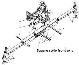
Versions were also made with an additional stay rod to make the whole assembly stronger, but this style isn't very common.
