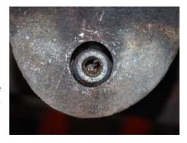
To give an example of how tight this pin can stick with this level of neglect, this photograph shows the casting and axle in a 30 ton press where the pin still wouldn't move. Eventually it took a 50 kW gas torch to heat the centre of the axle while at the limit of the press before it would move.
