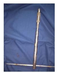
usually glass hard. You can push the reamer in and out (hand force only) when preparing to take a new cut – I tend to go for 1 or 2 thou at a time adjusting and measuring across the cutters with a micrometer, not a vernier caliper, for accuracy. When you've finished with the reamer, oil or grease it and wrap in oil-paper of cling film to protect the edges from damage and rust.
