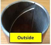
Read that article for suggestions on how to remove the axle bushes. If you use a tap, a 1-1/4" UNF or UNC taper tap works well. The bush may need reaming – some do but not all depending on supplier.
